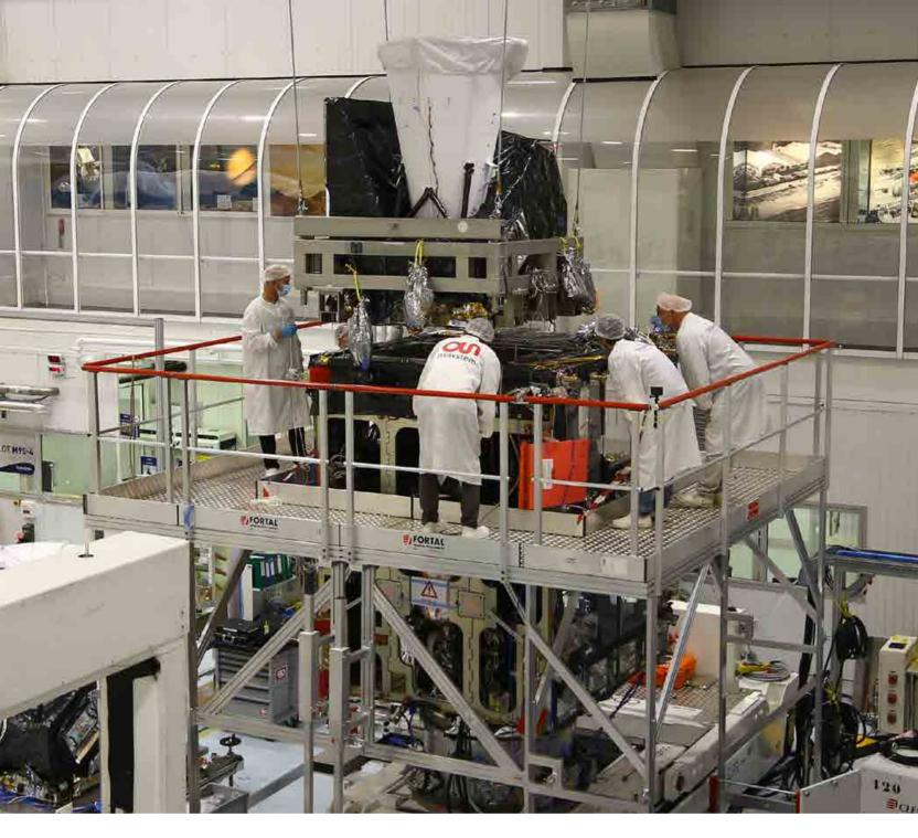
After completion of the first flight model of the Flexible Combined Imager in July 2021, the instrument is successfully mounted on to the MTG-I protoflight platform (credit: Thales Alenia Space)
