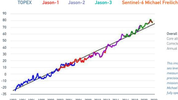
**Overall trend: 3.29 mm/yr** Core altimeters up to 66<sup>0</sup> latitude Corrected for GIA Annual signal removed
