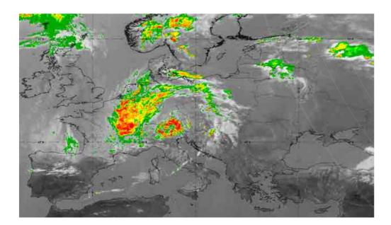
The slow-moving nature of the storm in the image, left, led to significant accumulations of rainfall and devastating flooding. The areas of most intense rainfall are shown in red. The image uses the Nowcasting Satellite Application Facility's precipitating clouds product overlaid on a Meteosat infrared 10.8 micron image and was taken on 14 July 2021.
