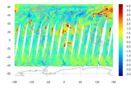
Absorbing aerosol index using polarisation measurement devices data collected using Metop-C's Global Ozone Monitoring Experiment-2 on 12 August 2021
